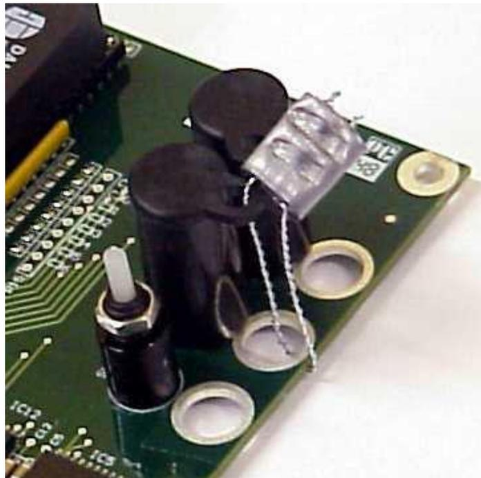
Typical Sealing of Meter Calibration (k-factor) Switch
