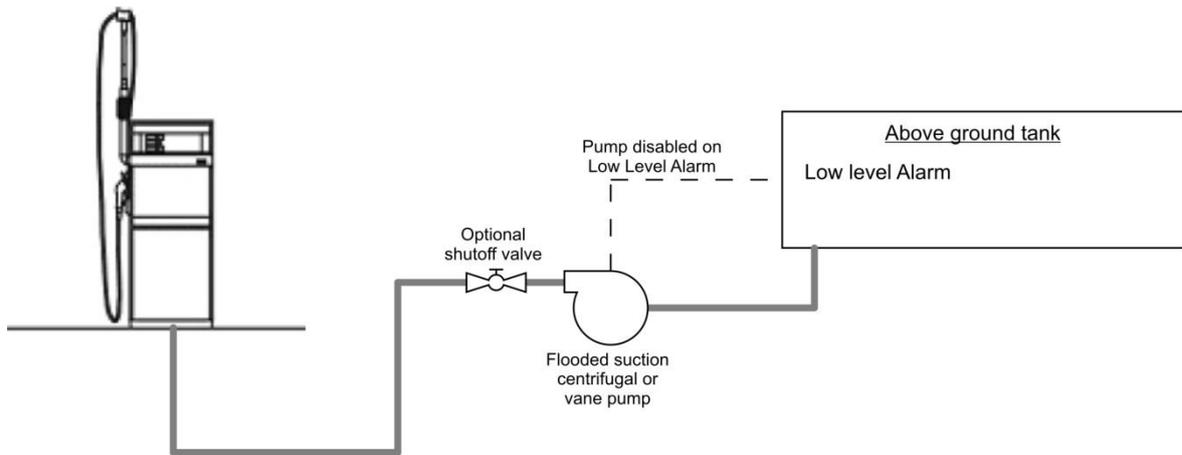
(a) Compac Model MA30S (AdBlue) Liquid Dispenser – Typical Installation
