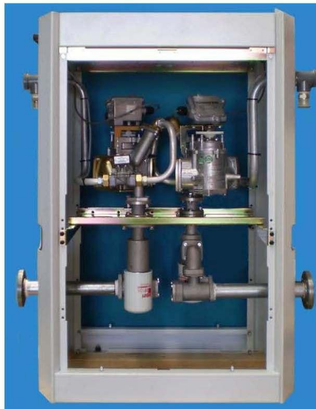
Typical 801 Series Fuel Dispenser (2 inlet/2 outlet, with and without covers) – Variant 2
