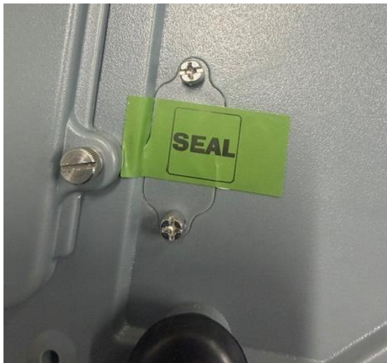
(b) Cover Plate Sealed with Destructible Adhesive Label
