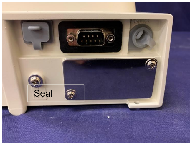
(b) Sealing Arrangement Using Destructible Adhesive Label
