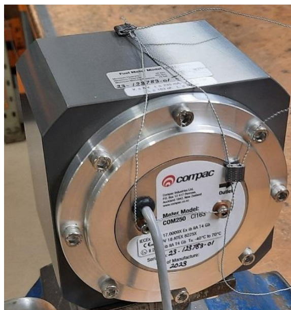
Compac COM 250 flowmeter with anodised aluminium housing (Variant 5)
