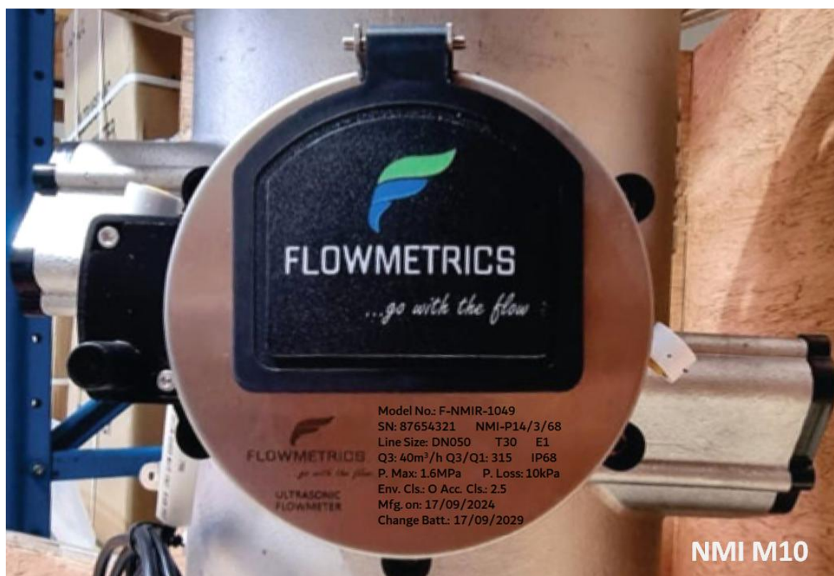
Example of required markings – Accuracy class 2.5
