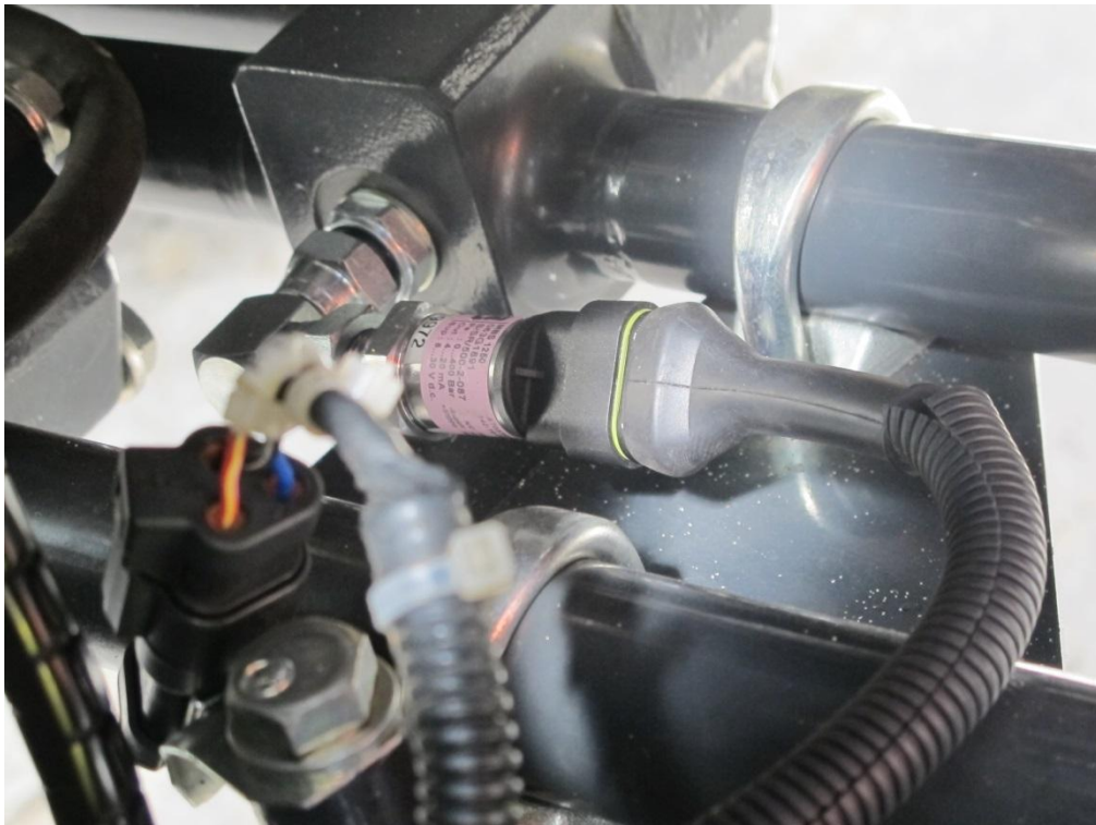
Typical RDS Pressure Sensor Installation
