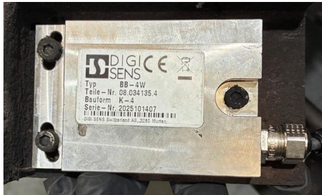
(a) DIGI SENS AG Model Type BB Accelerometer Sensor
