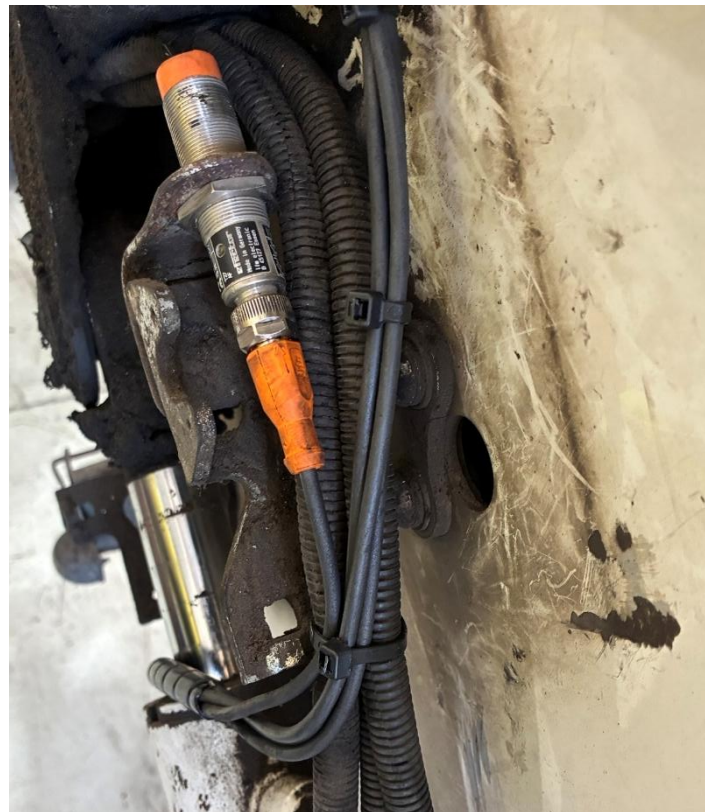
(b) Ifm Electronic Model IG5597 Inductive Sensor Located to Define Measuring Window
