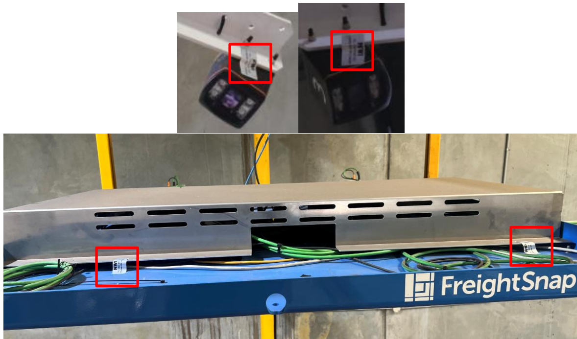
b) Typical Mechanical Sealing Provision on the FS-5000 (Variant 2)
