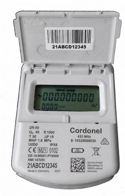
Example of required markings
