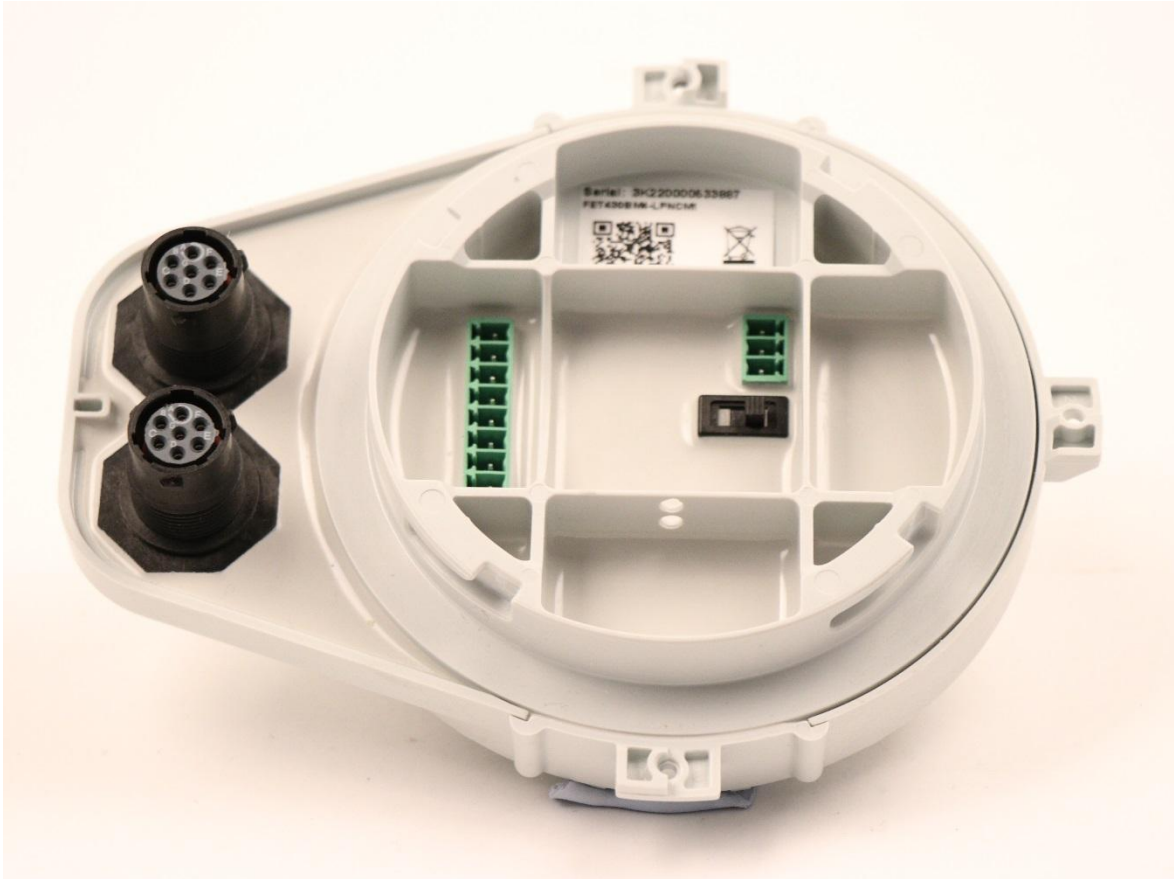
AquaMaster4 – Sealing Device: read-only switch
