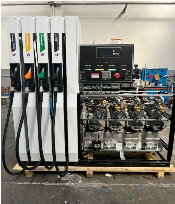
Mithra Fueling Model INNO 6000 L 482-S Fuel Dispenser Hydraulics (Suction Type with vapour recovery components)
