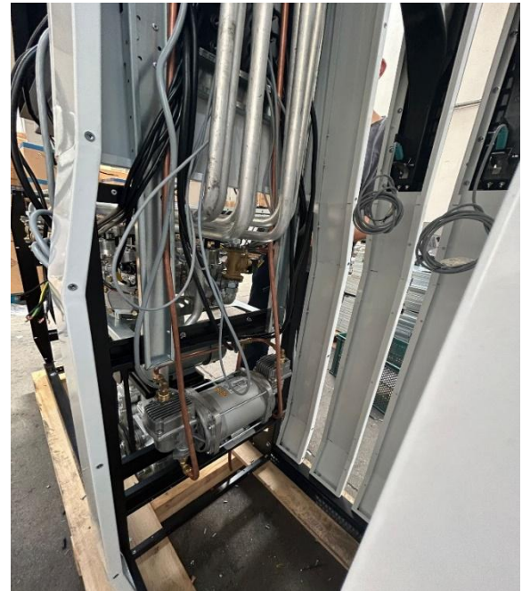
Mithra Fueling Model INNO 6000 L 482-S Fuel Dispenser Hydraulics (Suction Type with vapour recovery components)
