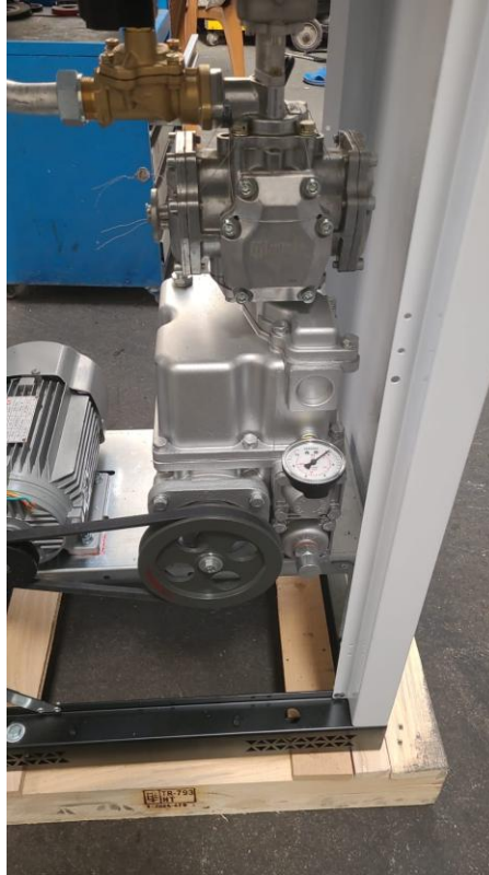
a. Fuel Dispenser Hydraulics
