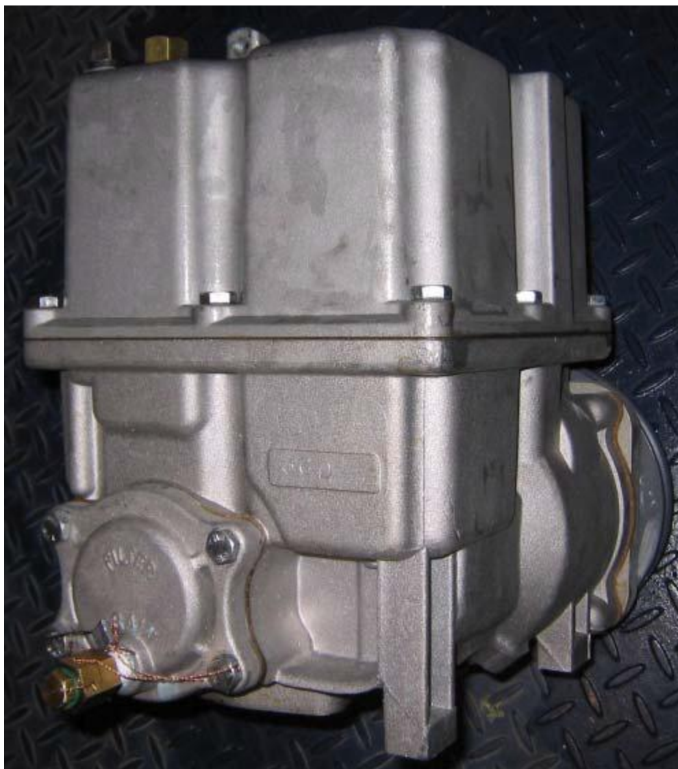
Showing Typical Sealing of Gas Elimination Device Air Test Valve Access Point
