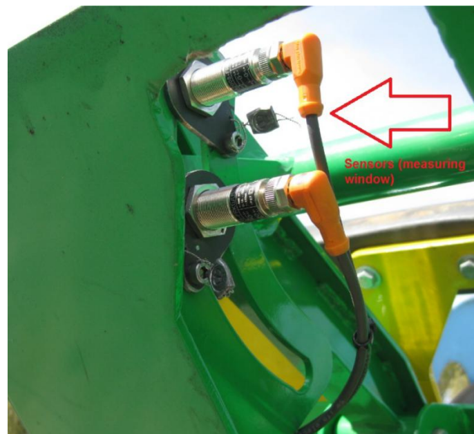
(b) Sensors Located to Define Measuring Window
