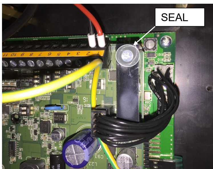
Typical Sealing of Protective Cover
