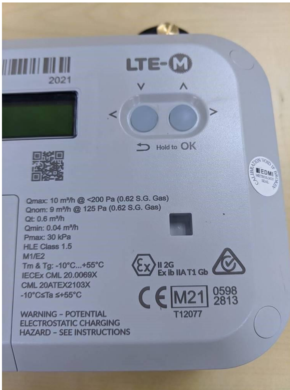
Example of required markings
