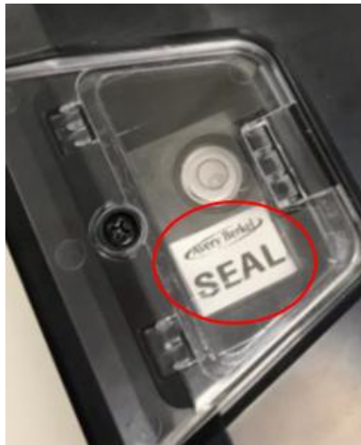
Typical Sealing of X-Pro Series Instruments with Destructible Adhesive Label (Sealing provision)
