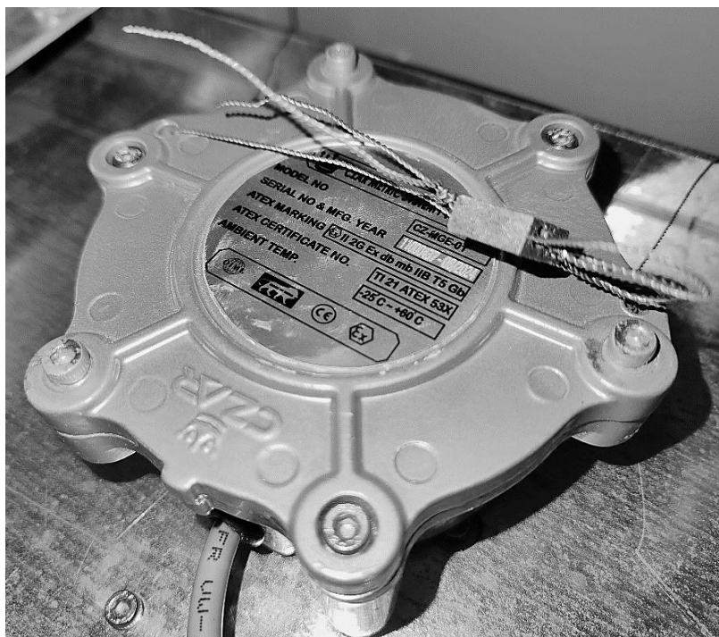
CZAR model CZ-MGE-XX Magnetic Pulser with sealing method.
