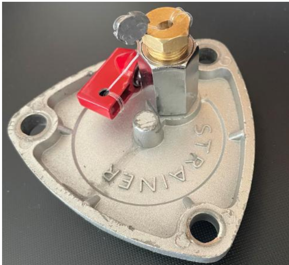
For all models Manufactured before June 2023 - Typical Sealing of Air separation test valve
