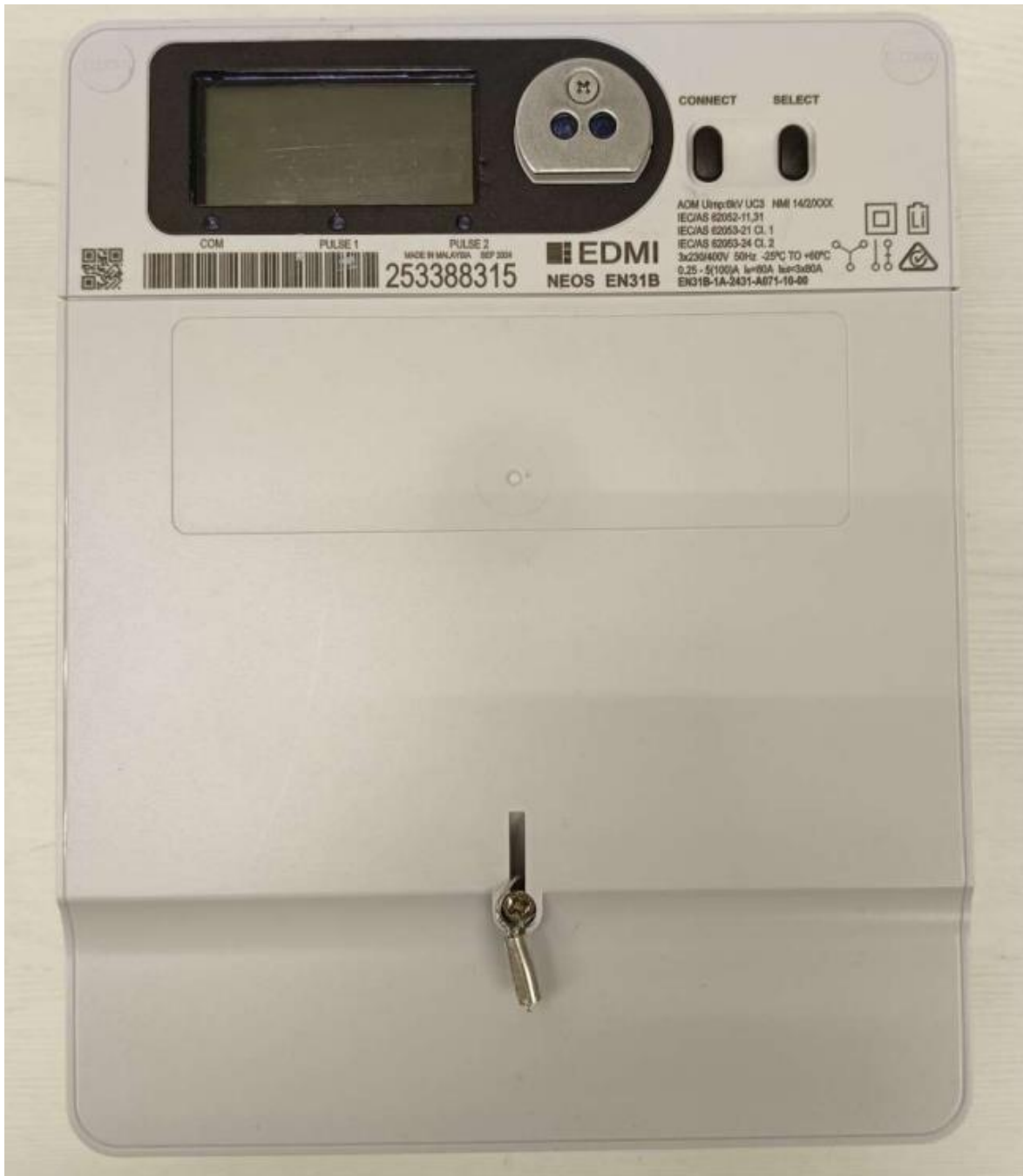
EDMI Pty Ltd model NEOS EN31B Class 1 Electricity Meter (the pattern, including Typical Mechanical Sealing)
