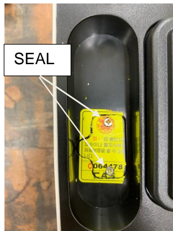
(a) Lead and Wire Type of Seal
