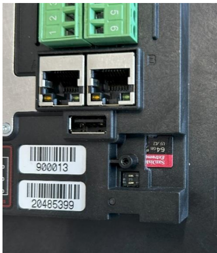
Location of calibration microswitch with and without cover Variant –3
