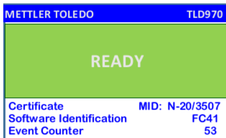
(a) Sealing and Event counter displayed on CS220 USB display
