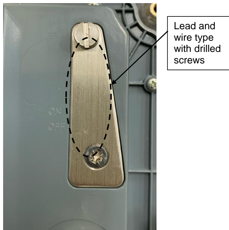
Sealing of i-DT61PW Digital Indicator
