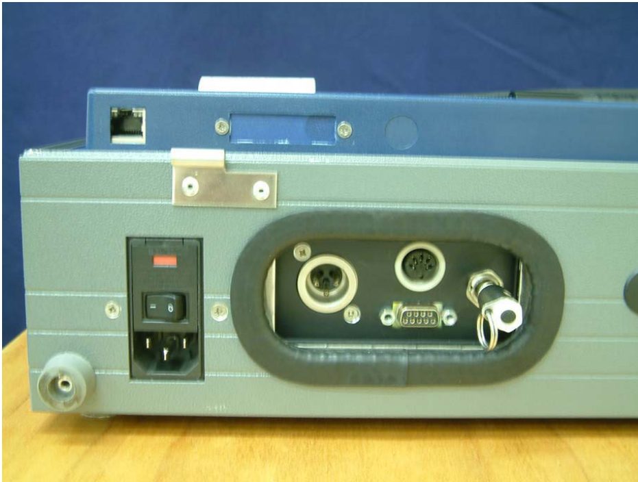
Showing a Typical Ethernet Port (Variant 1)
