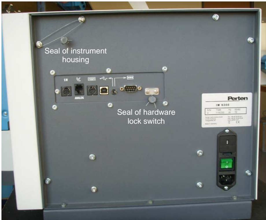
(a) Typical Sealing of Perten Inframatic IM9200 (lead and wire type seal)
