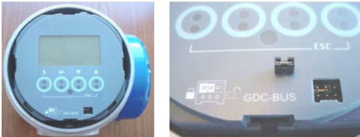
Sealing arrangements - Weights and Measures jumper
