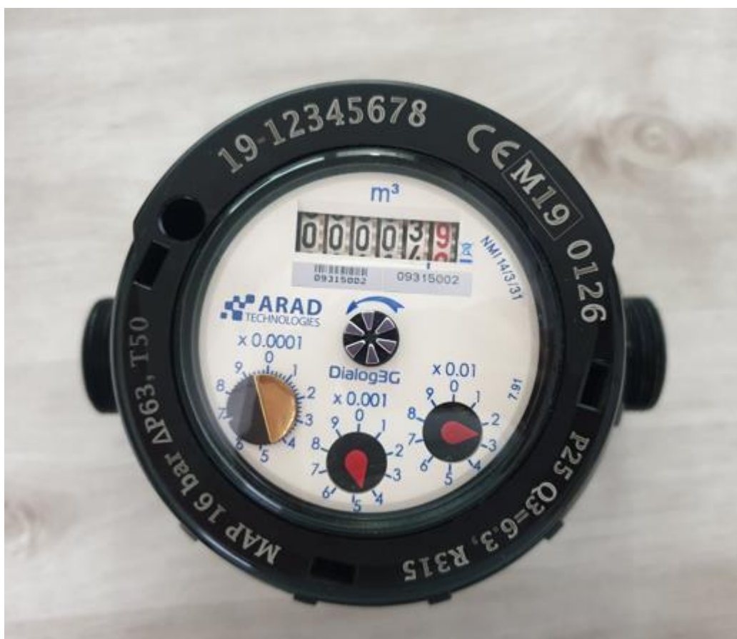
Mechanical register with electronic 3G unit – Variant 3
