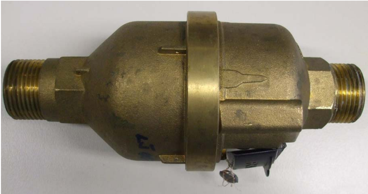
(a) Model WM210 PD Water Meter (including flow direction indication)
