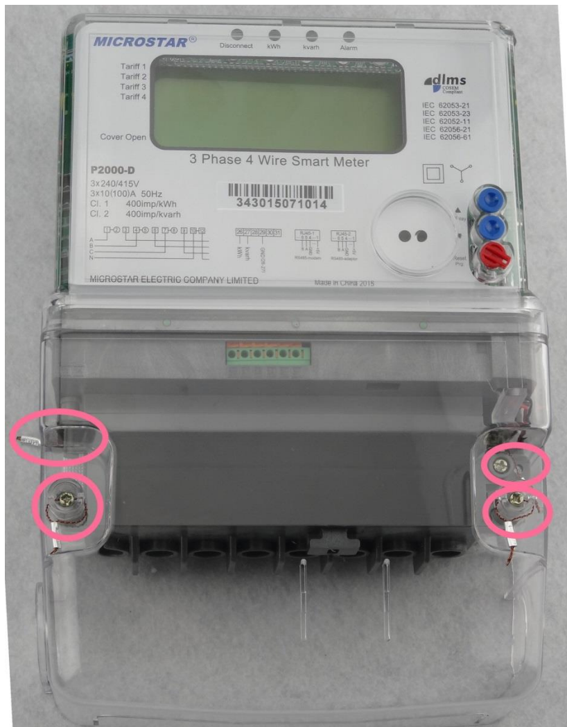
Microstar Model P2000-D (Including Typical Mechanical Sealing)
