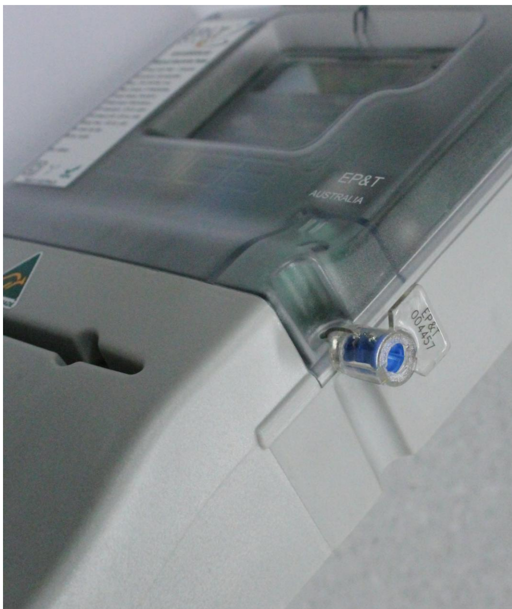
Typical Mechanical Sealing of Model Edge g3
