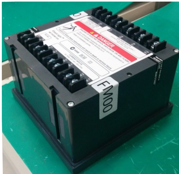
Showing Typical Sealing Method – Destructible Labels in at Least 2 Locations
