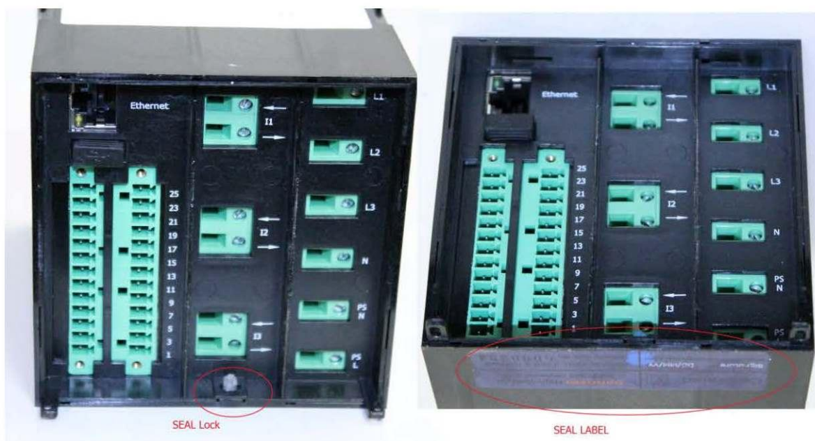
EP&T Model Edge g6 MBC Electricity Meter (Including Typical Mechanical Sealing)
