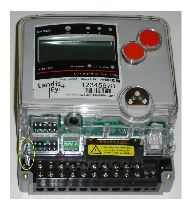
Landis+Gyr Model EM5300 Class 0.5 Electricity Meter (Including Typical Mechanical Sealing)
