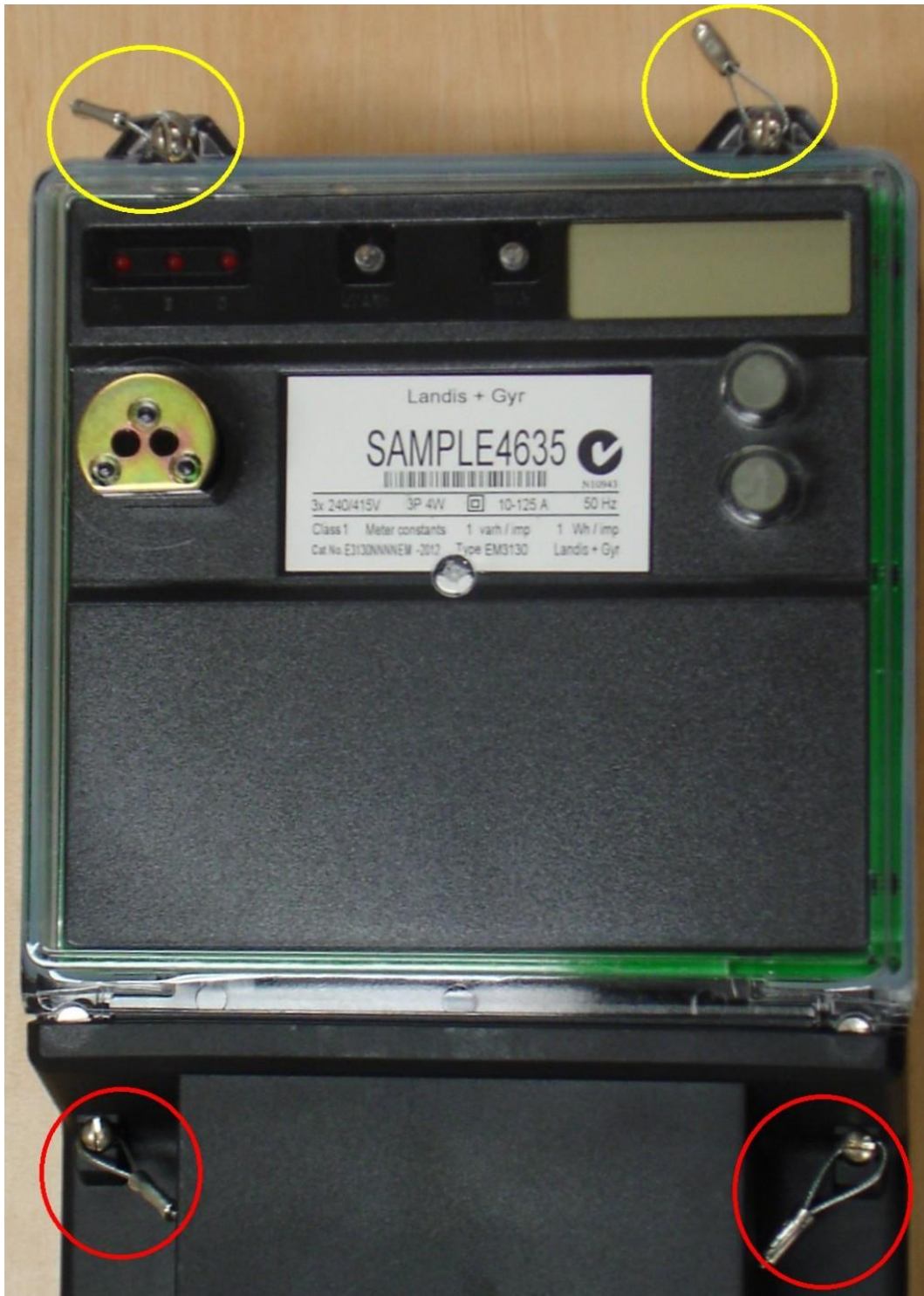
Landis+Gyr Model EM3130 Class 1 Electricity Meter (Including Typical Mechanical Sealing)
