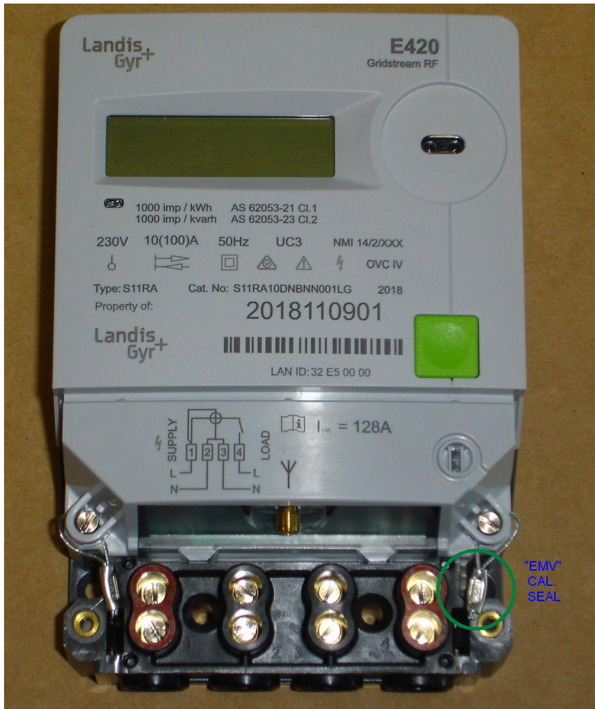
Landis+Gyr Pty Ltd model E420 S11RA Electricity Meter (The Pattern) including typical mechanical sealing.
