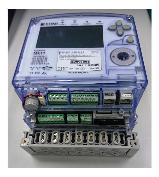
EDMI model Genius Mk11 CT Electricity Meter displaying terminal connections
