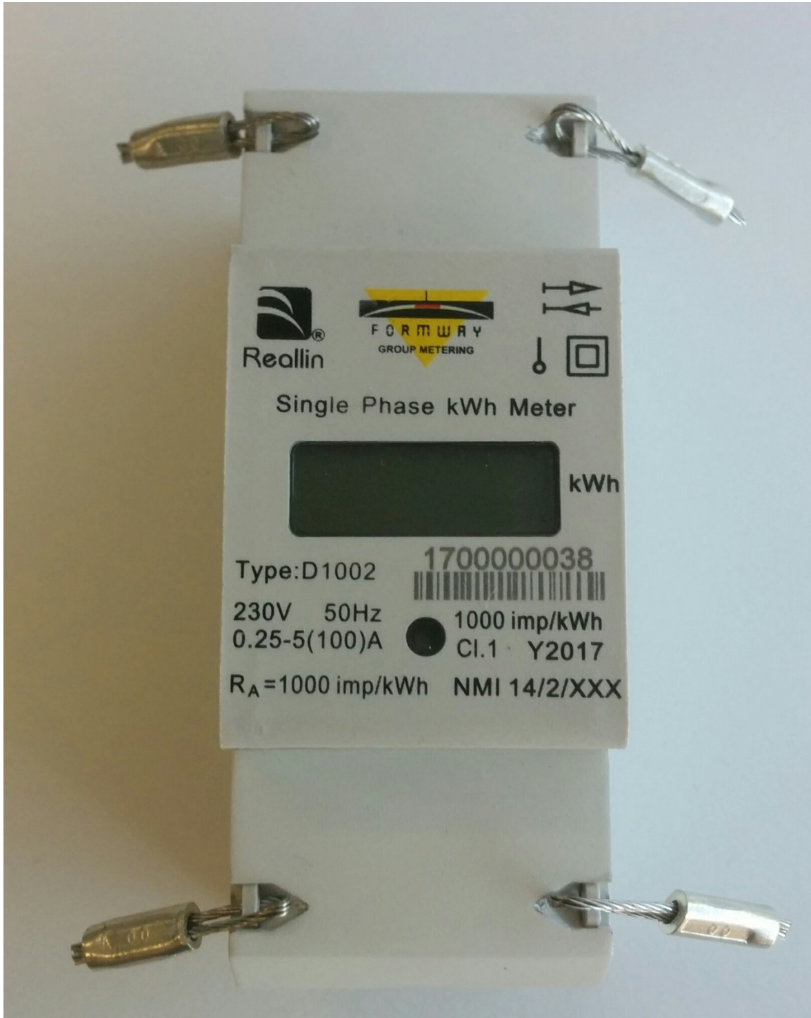
Typical Mechanical Sealing
