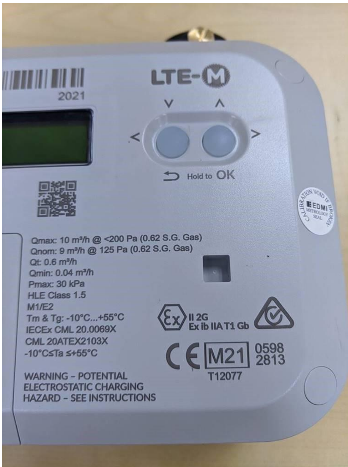
Example of required markings
