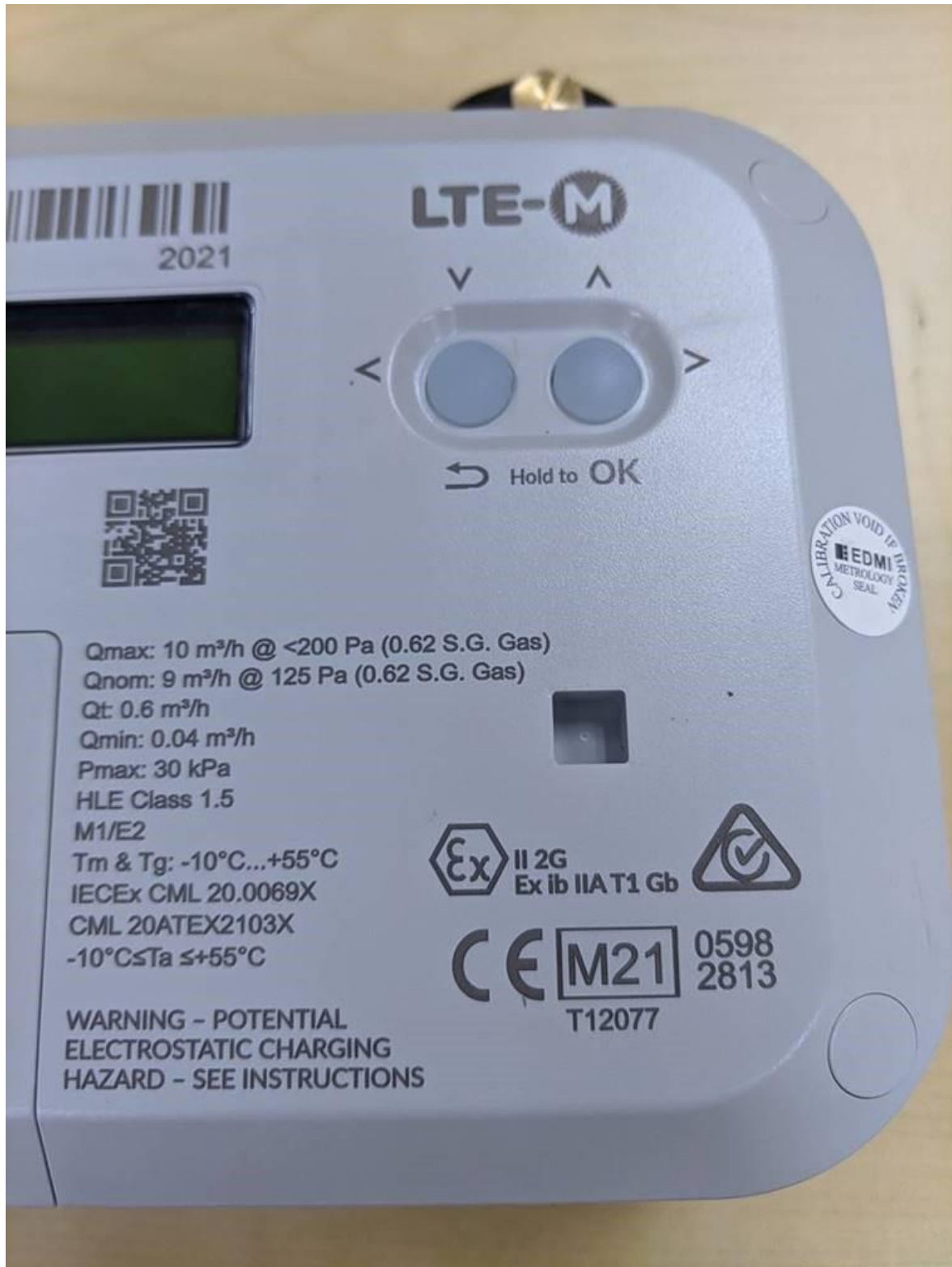
Example of required markings
