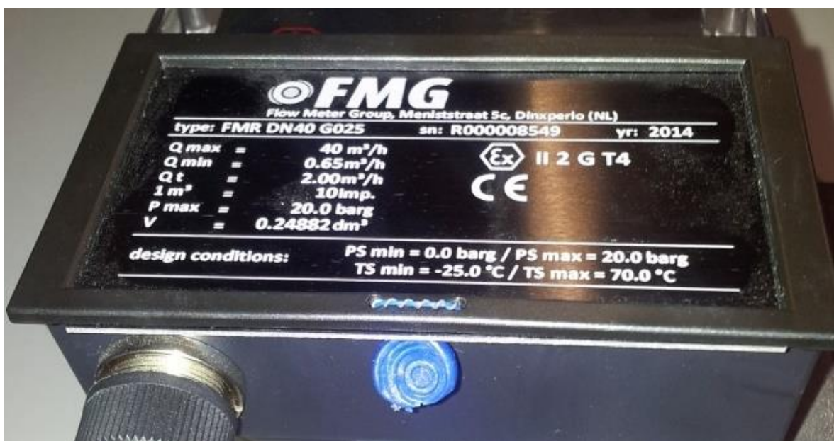
(b) Typical Sealing of Indicator (Note markings shown are NOT correct for Australia)
