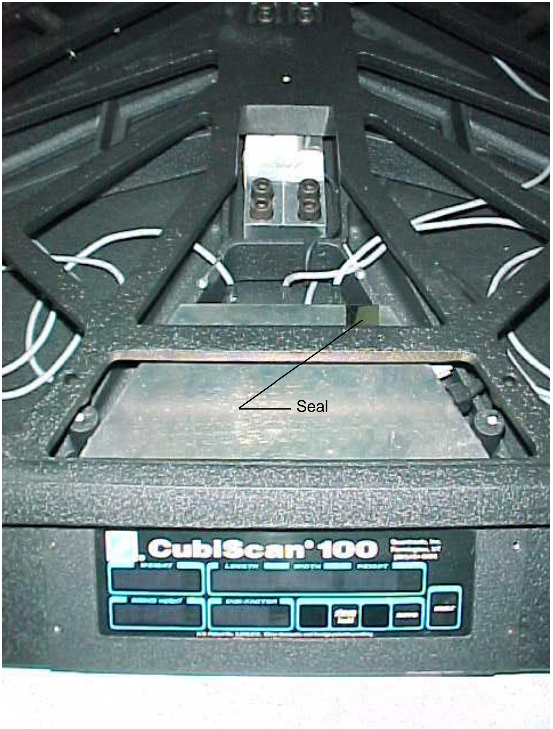
Showing Load cell Mounting and Controller Box Sealing
