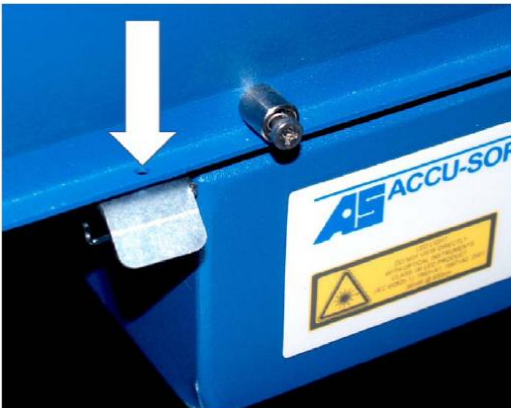
Showing Typical Mechanical Sealing Provision on the Camera Module
