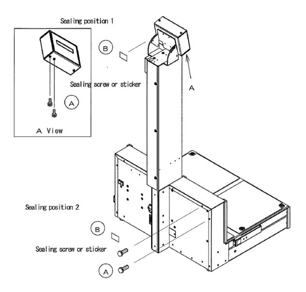
Showing Typical Sealing of Model SPK-1000 Instrument
