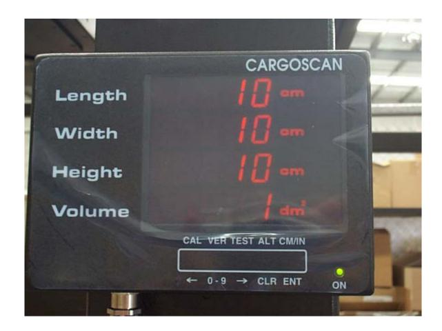
Cargoscan Model CS2200 Indicator/Control Panel
