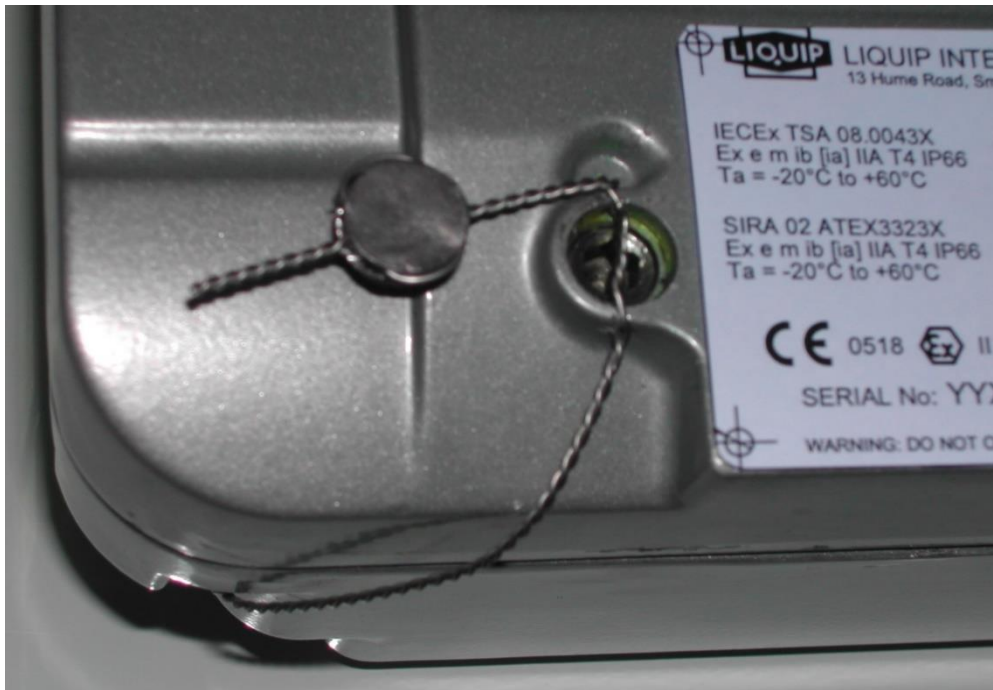
Typical Sealing of the CAL Button to a cover-mounting screw (not shown)
