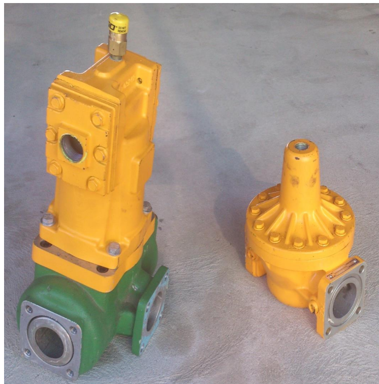
(b) Liquid Controls Model MA8310 Gas Extractor and Liquid Controls Model A 2843 Differential Pressure Valve
