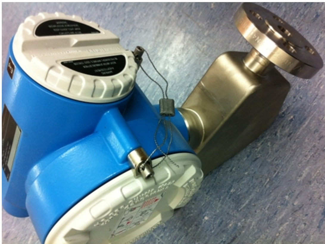
A Typical Sealing Method – Endress+Hauser LPG Meter – The Pattern
