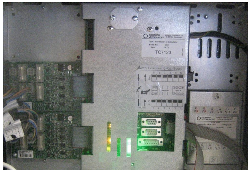
Processor PCB and Interface Cards
