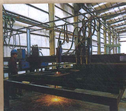
仿形切割機 Cutting machine of profile moldeelling
