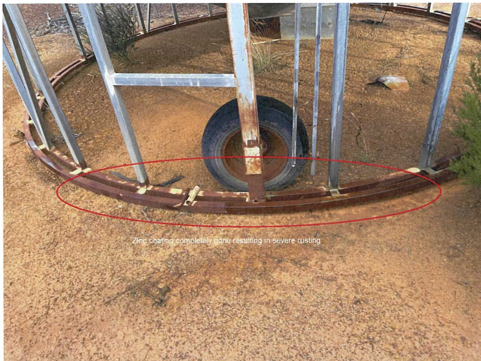
Picture 7. This picture is a close up of rusted Duragal® silo stand.
